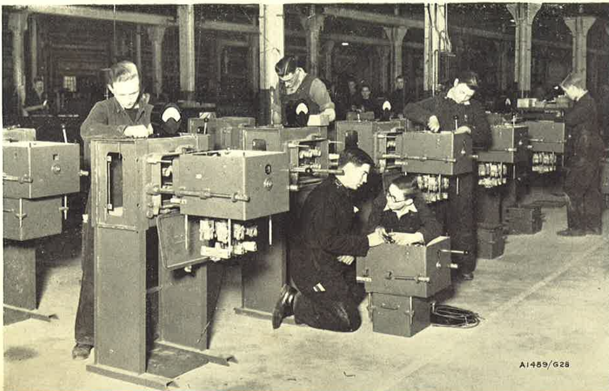
Above :—Apprentices assembling 400 ampere horizontal isolation type switchgear.
