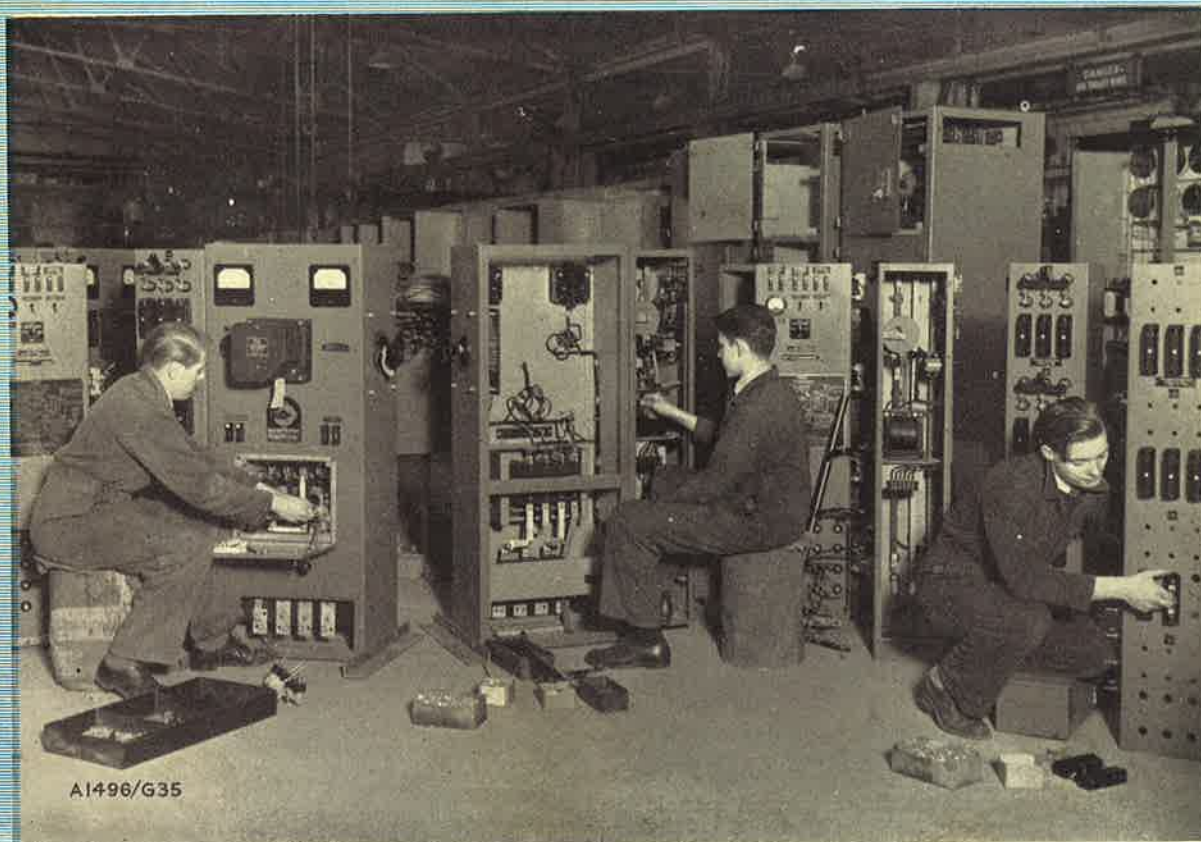
Below :—Apprentices assembling control panels for 55 kilowatt diesel driven generating sets.
