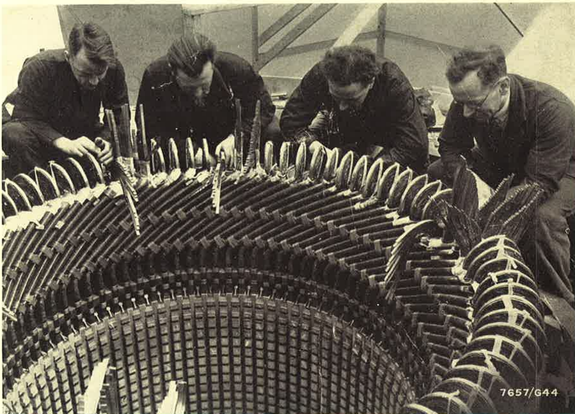
Graduate Apprentices assisting to connect the ends of the stator windings of a 30,000 kilowatt Turbo-Alternator.
