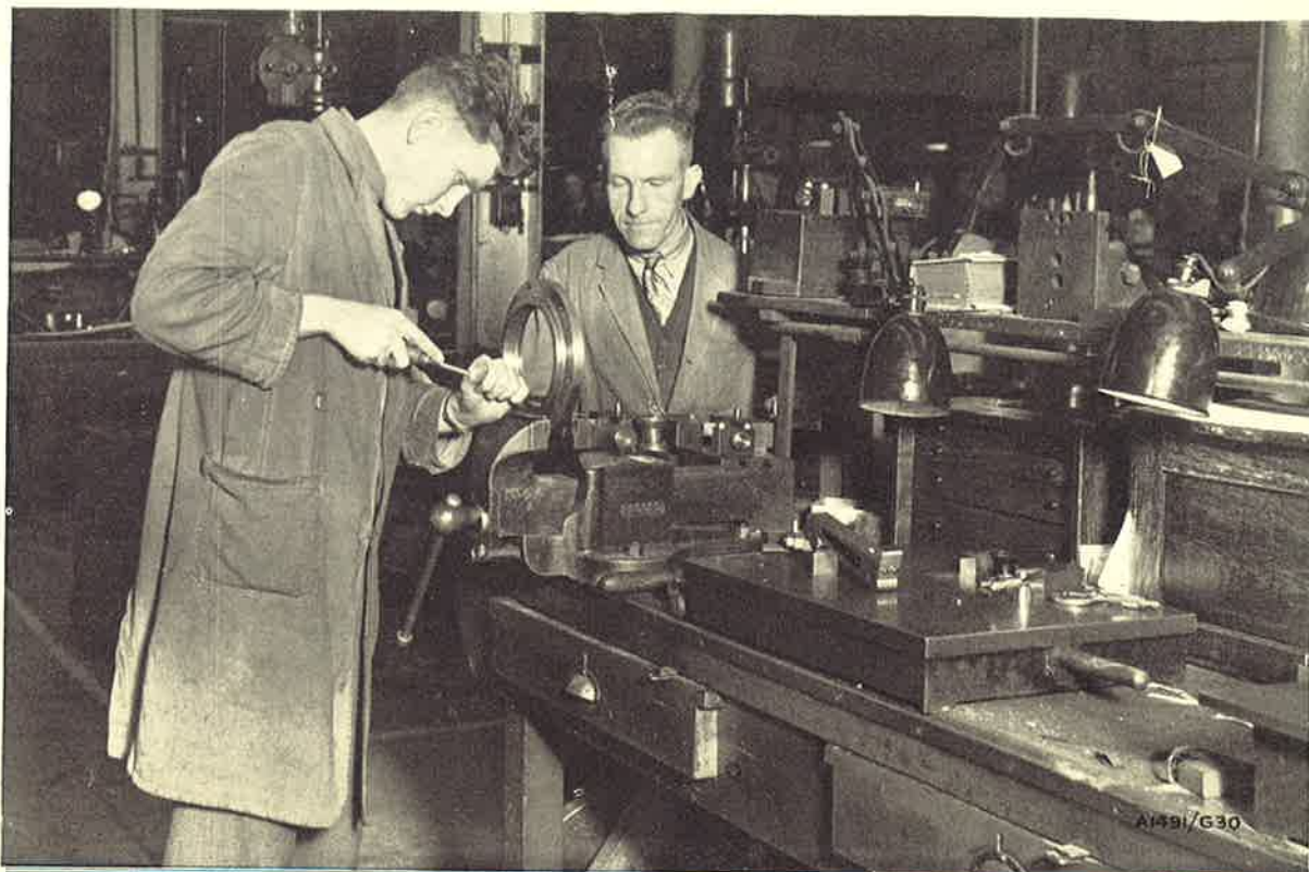
An Apprentice Tool Room Fitter scraping the bore of a coupling plate.
