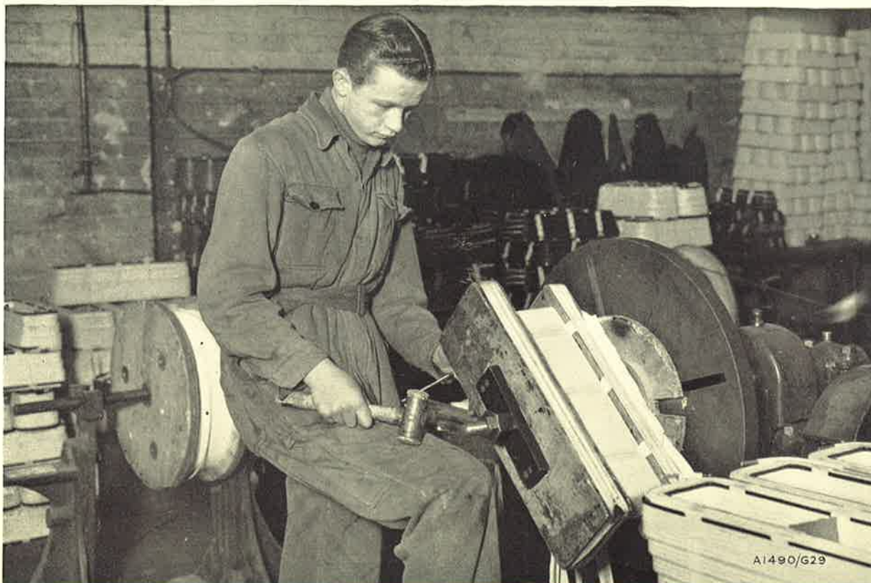
(Above) Winding rotor coils for 400 kilowatt Alternators.
